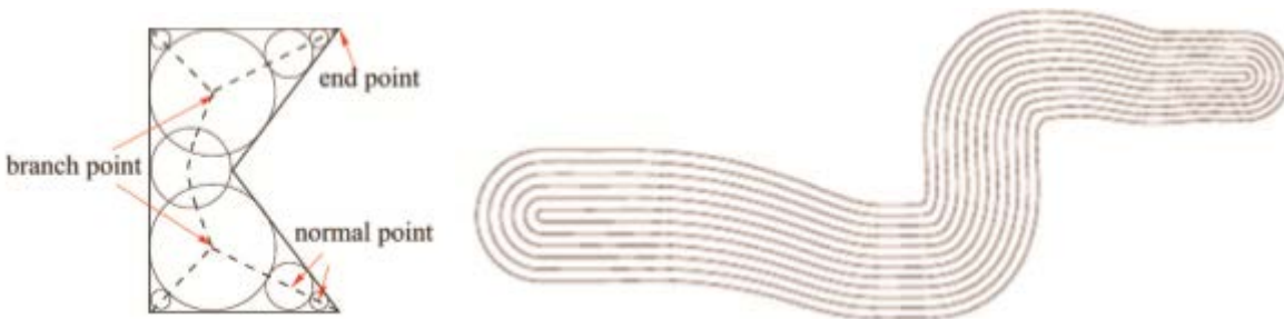
Figure 4. Medial Axis Transformation concepts and application in tool path planning
